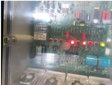
Figure 1: Counting trip counts during annual routine maintenance
